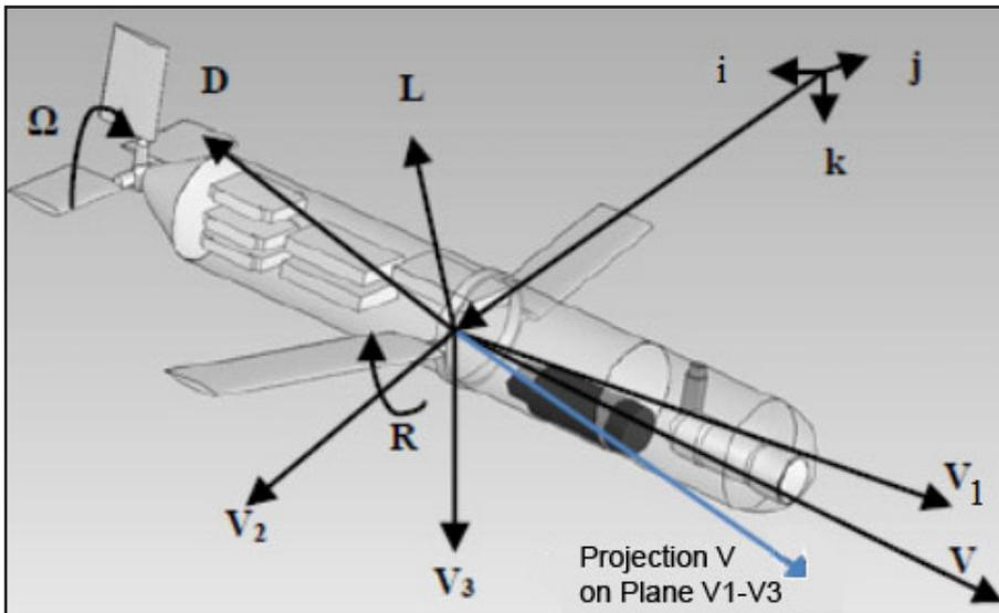
Figure 1. The dynamic forces of the glider.
