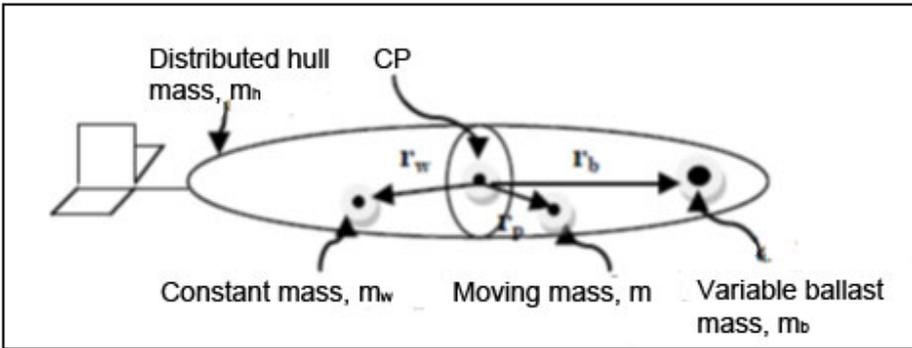
Figure 2. Defining of the underwater glider masses
