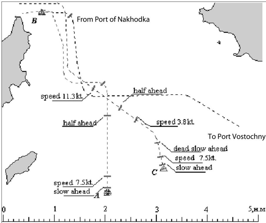
Figure 1.1. Situation with the vessels A, B, C in gulf of Nakhodka and advisory on maneuvering
