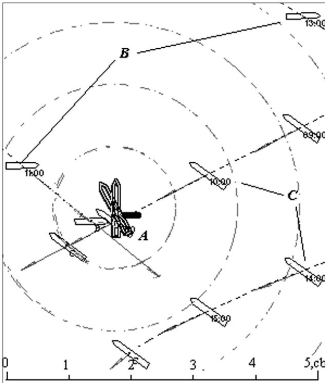
Figure 1.2. Superimposition of relative traces of vessels B, C relatively to vessel A while proceeding according to the advisories and in a case if no appropriate actions to be performed.
