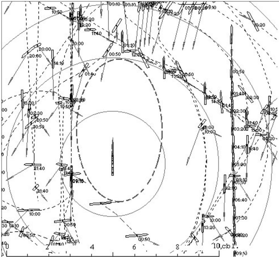
Figure 2.2. Superimposition of the relative traces of the all 9 vessels in course oriented datum
