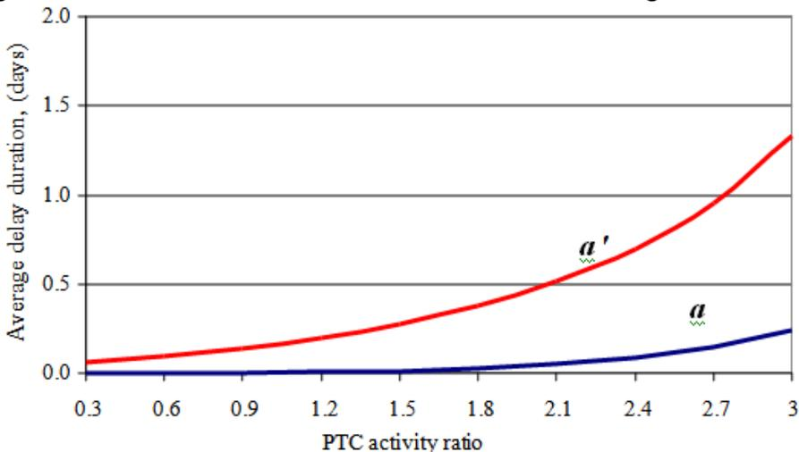
Figure 3. Delays of vessels waiting the processing with two options of workforce assignment in the port.
